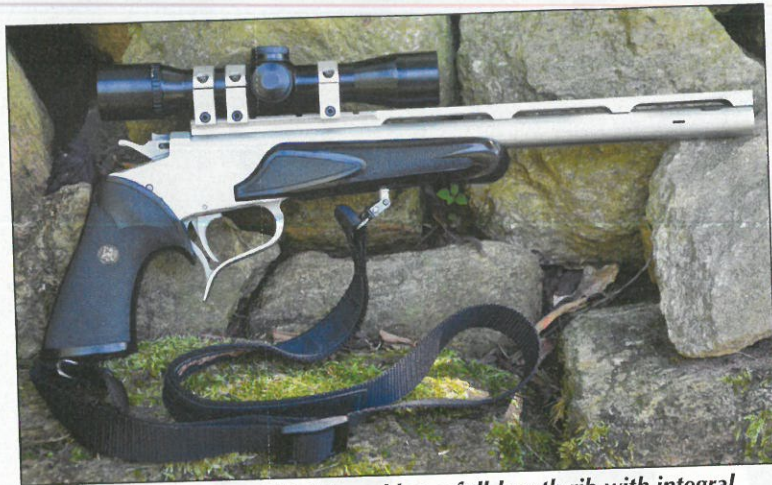
Layne's 14-inch SSK .375 JDJ barrel has a full-length rib with integral T'SOB scope mounting base. It is shown here with one of a limited run of Contender "flat-side" (no etching) frames, Pachmayr rubber grip and forearm, quick-detachable carrying sling and a Bausch & Lomb 2x handgrip scope.
