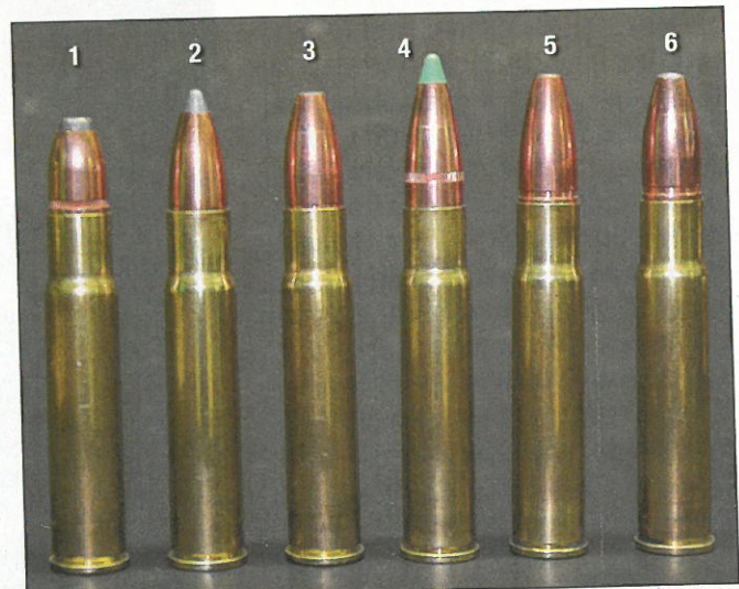
The .375 JDJ chamber throat is long enough to seat bullets with their bases no deeper in the case than the shoulder/neck junction: (1) Sierra 200-grain FN, (2) Sierra 250-grain SBT, (3) Swift 250-grain A-Frame, (4) Nosler 260-grain Ballistic Tip, (5) Swift 270-grain A-Frame, (6) Swift 270-grain A-frame.
