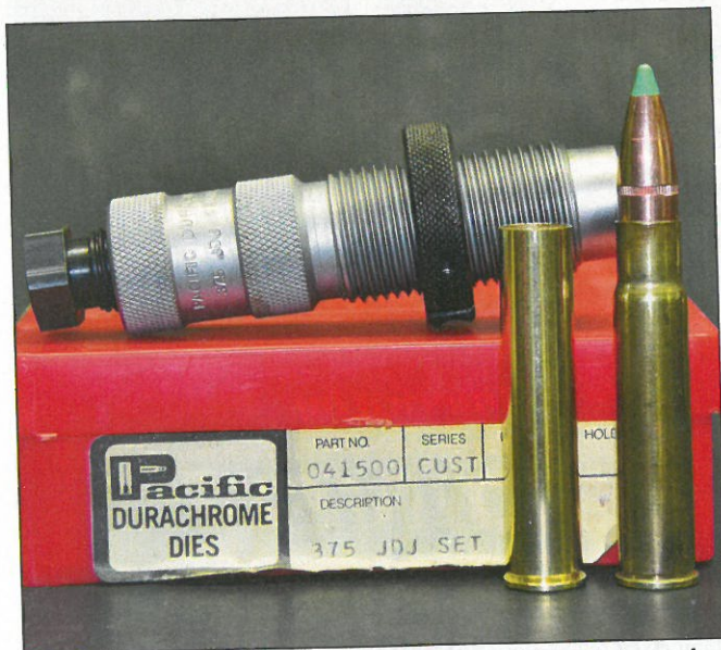
Cases are formed by using a full-length resizing die to neck down the .444 Marlin case (left) and fireforming to the .375 JDJ shape (right).
